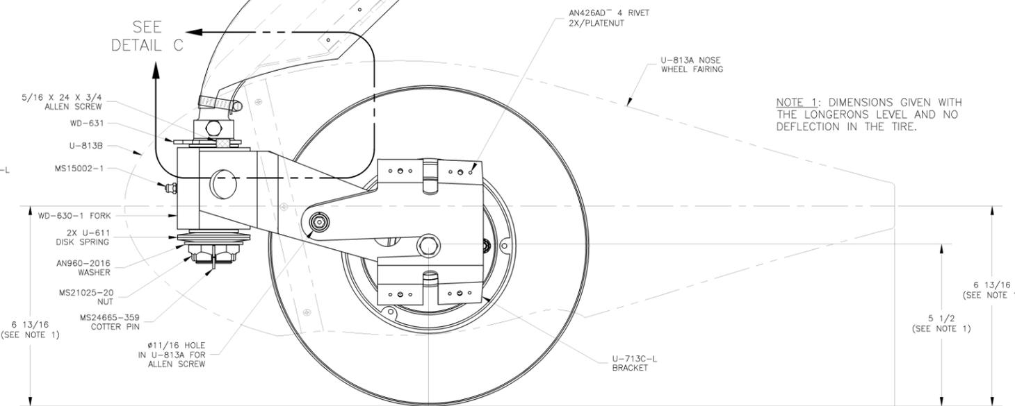
NOTE 1: DIMENSIONS GIVEN WITH THE LONGERONS LEVEL AND NO DEFLECTION IN THE TIRE.
