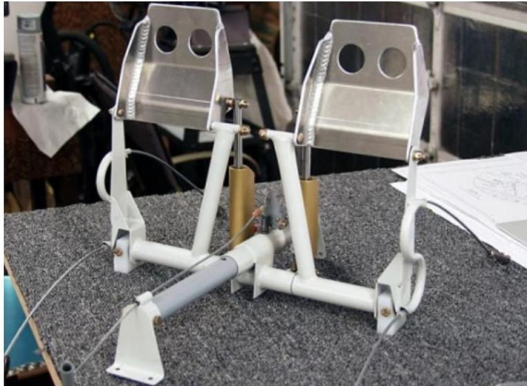
Rudder Pedals and Pivot Tubes
