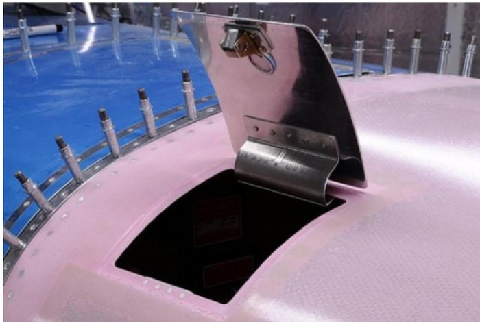
Sheet metal door installed after hole preparation
