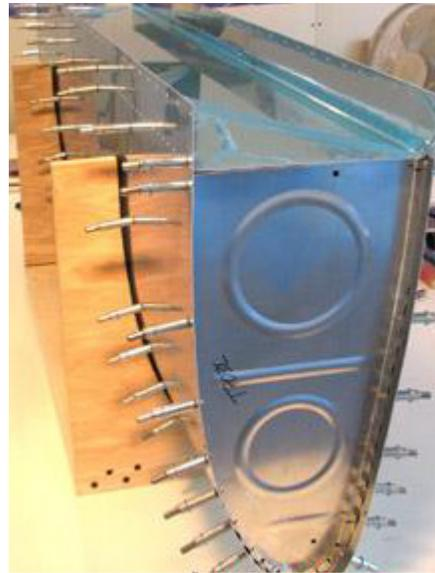
The outboard wing leading edge incorporates a fuel tank.
