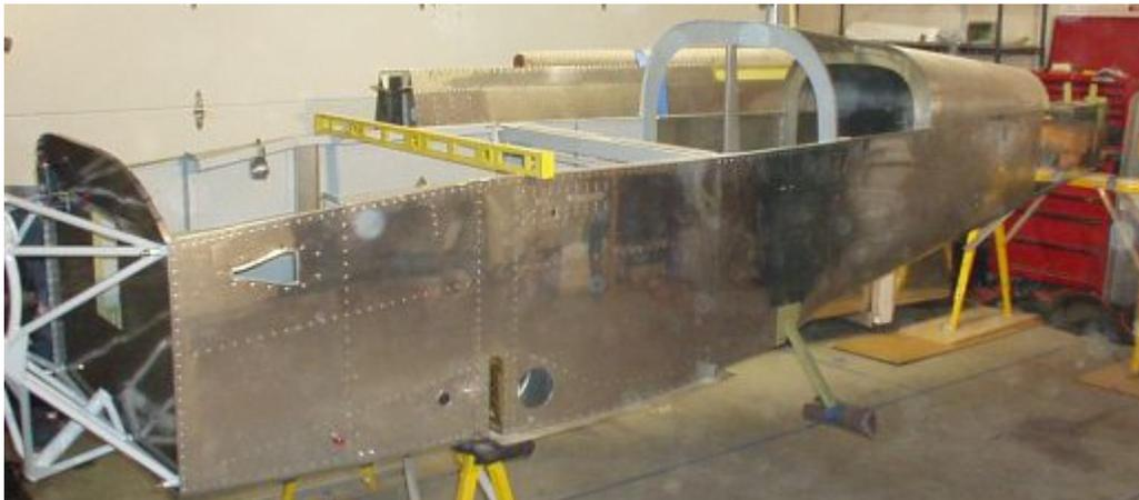
Quick build Kit Fuselage out of the crate
