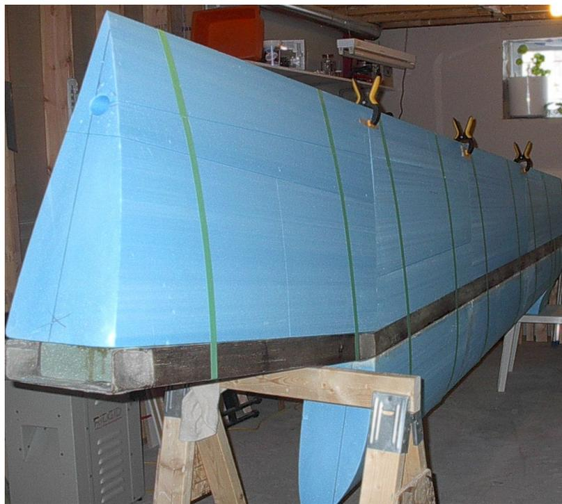
Wing Foam Core mated to carbon fiber spar
