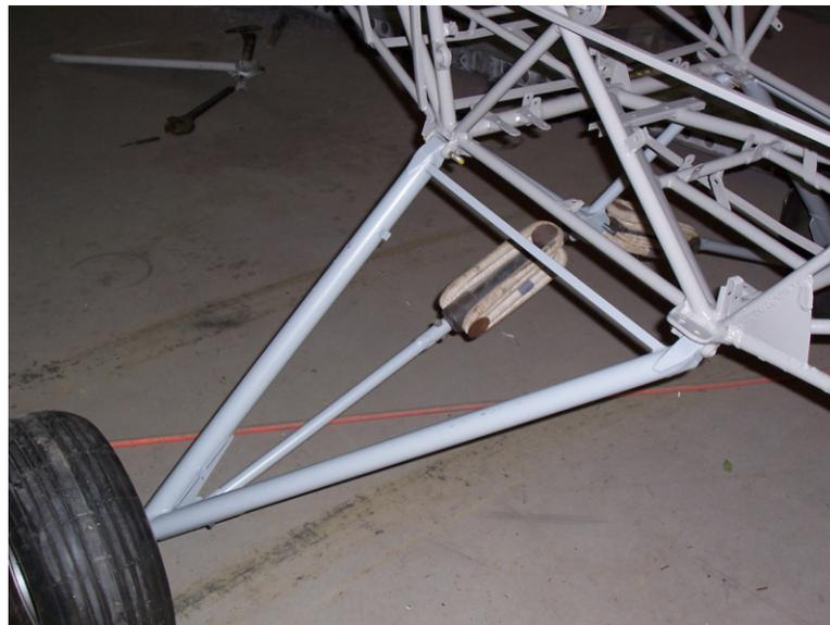
Steel Tube and bungee system used on Cub-like aircraft kits
