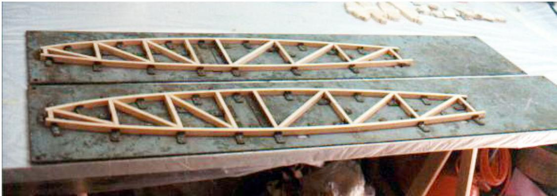
Ailerons constructed from plans and raw materials using a template/jig
