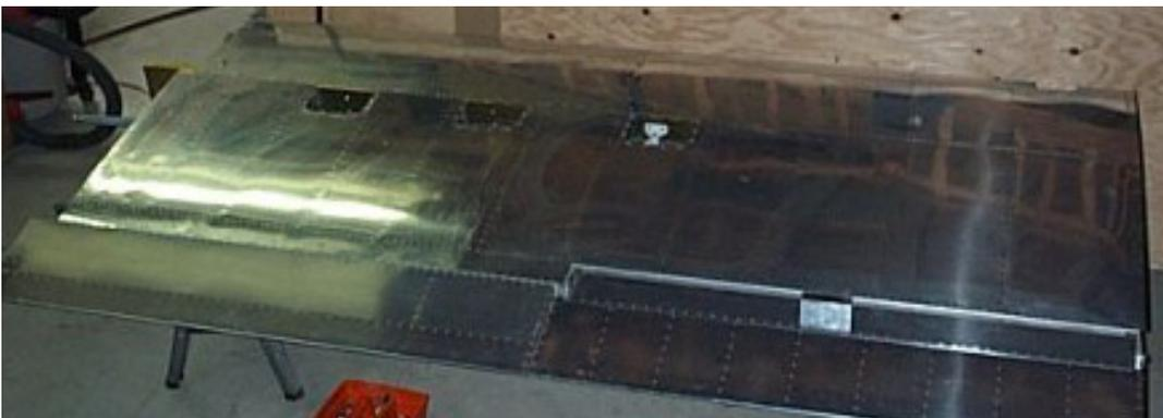
Completed Wing with Aileron and Flap attached
