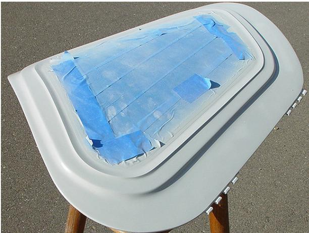
There are two fuselage window just behind the cockpit. Both are framed and fit to plexiglass. At least one has a hinge and latch mechanism for opening into the baggage area. The frames are cut and shaped by the manufacturer but require trimming, sanding, and bonding on both windows by the builder to complete the fabrication process. The scores may appear as such below.
