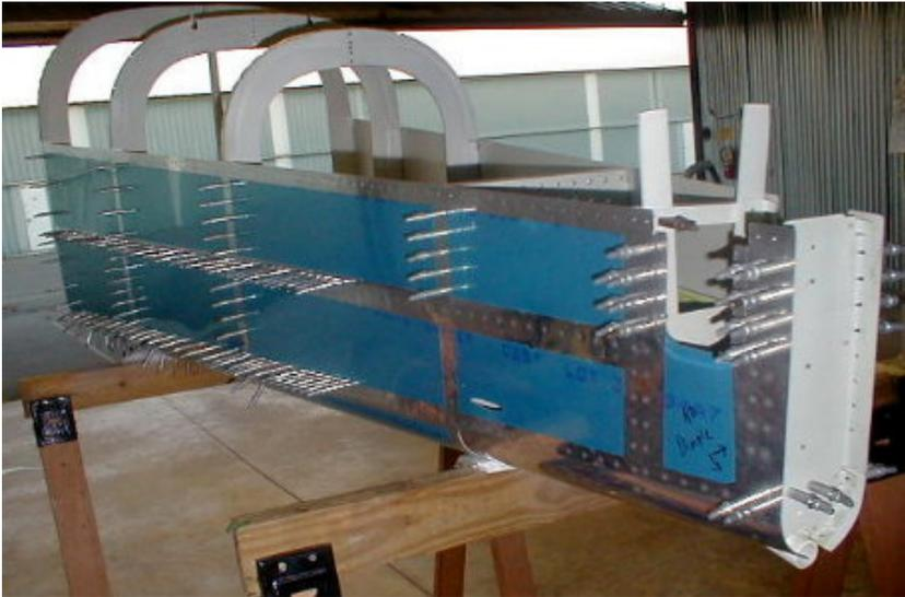
Aft Fuselage Section Standard Build Kit
