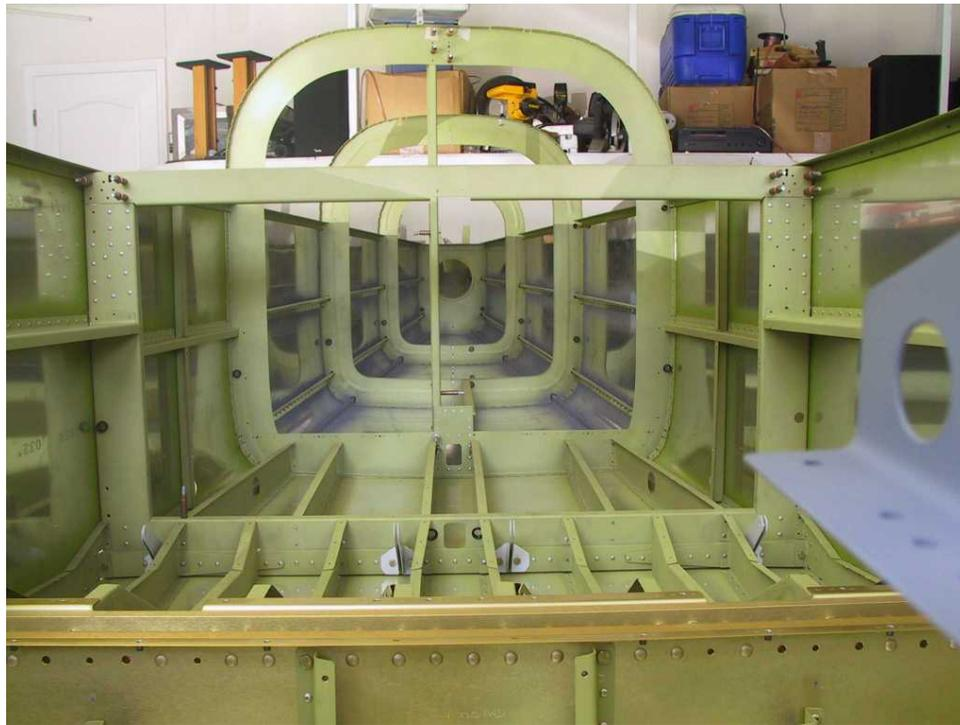
Standard Kit Fuselage structure assembled
