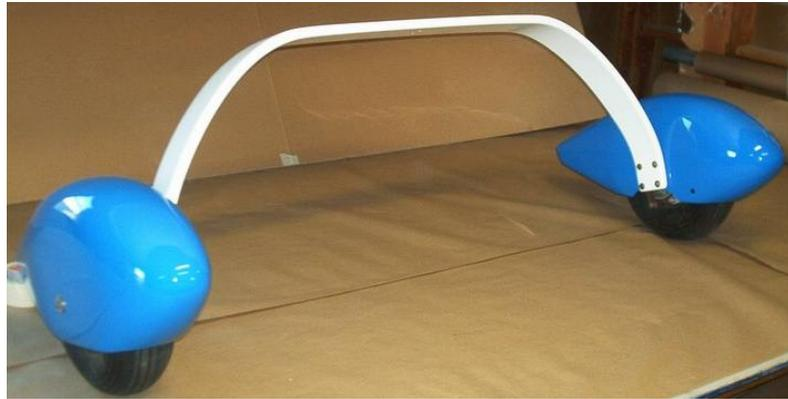
Composite (Carbon Fiber) Spring Landing Gear
