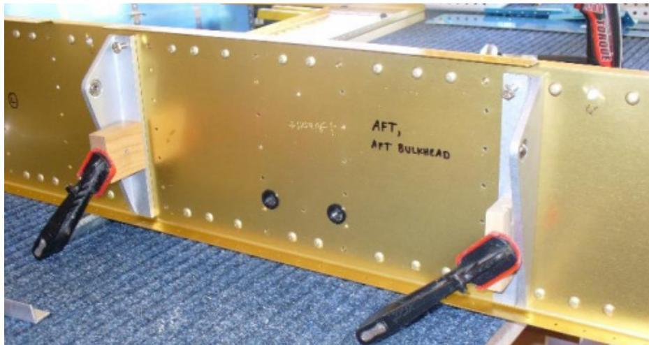
Typical Metal Bulkhead in a standard build kit
