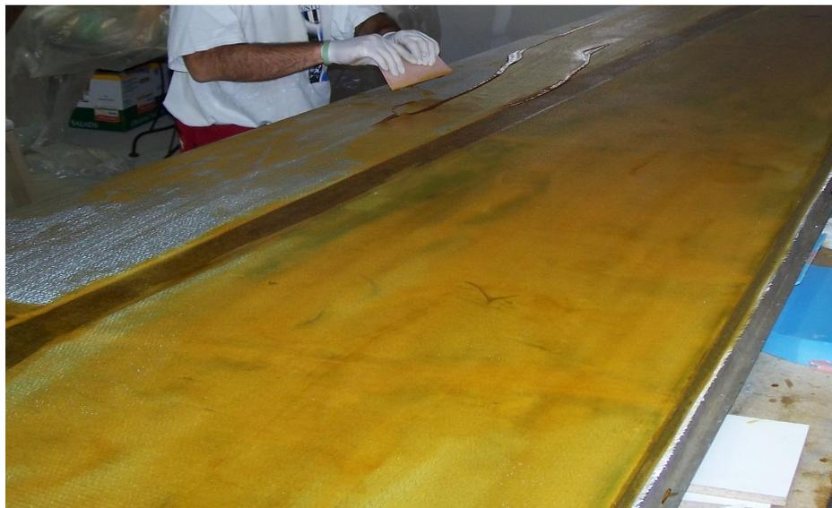
Applying resin to the fiberglass cloth to form composite skin
