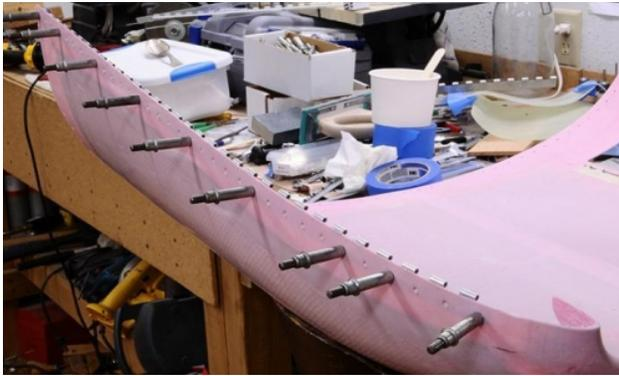
Composite cowling with hinge clecoed in place
