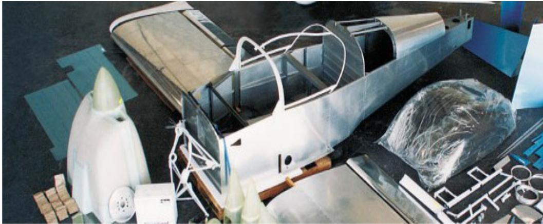
Quick build Kit with Quick build Fuselage
