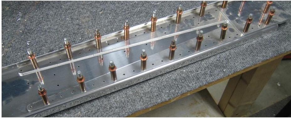
Wing Rear Spar with reinforcement plate in place with clecos
