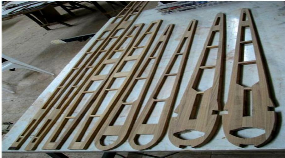
This photo shows horizontal stabilizer parts as provided by the factory. As such the builder will receive minor credit for fabrication.
