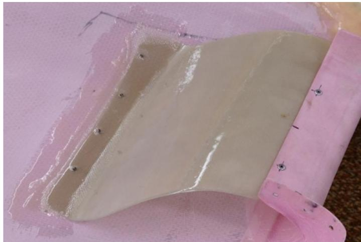
Inlet Duct molded to the Cowling
