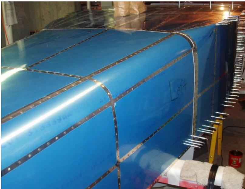
Skin panels being riveted in place on partially completed standard build fuselage structure. From the multiple rivet lines in this photo, numerous skin panels have to be prepared and attached to the fuselage structure, which translates into significant work for the builder.
