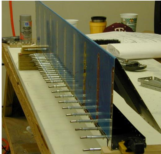
Aileron skin being joined to the aileron spar in task W25.
