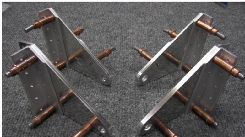
Aileron Brackets after trimming and drilling
