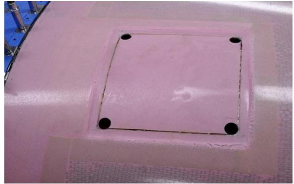
Composite cowling with door cut-out
