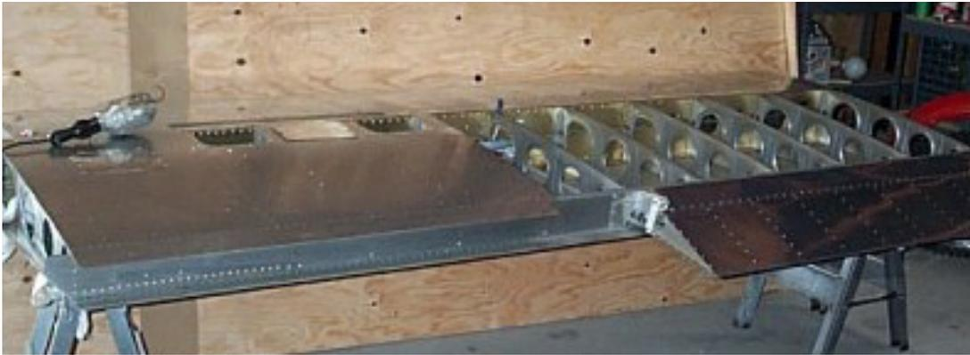
In the photo above, the aileron (fabricated and assembled at the factory) has been attached to the left wing (wing is upside down) by the builder.
