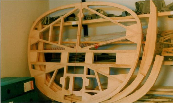
Here, the bulkhead is in an almost finished state, with just a few more braces needed for completion. With this photo and the photo above, the builder has some evidence to support the fabrication and assembly claims. However, these two photos don't prove that the internal components were fabricated from raw stock. The internal framing parts could have been included in the kit and the evaluator should pose the question on whether
