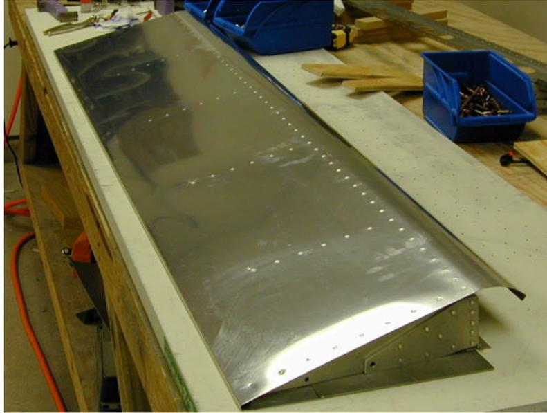
The flap on this aircraft does not have a conventional leading/trailing edge. The design extends the top flap skin past the spar in the front to cover the gap between the flap and wing. At trailing edge, the rear of the top skin folds down and under to overlap and then attach to the bottom skin.
