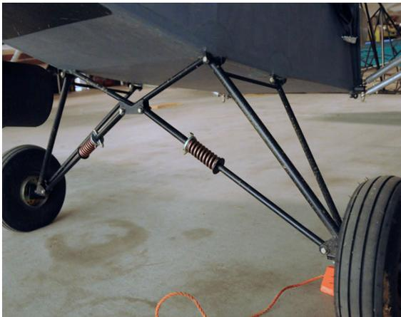
Spring and Steel Landing Gear
