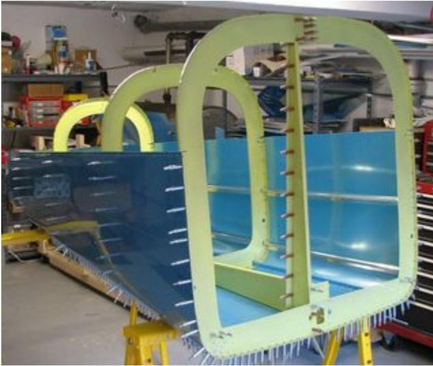
Aft Fuselage Section Standard Build Kit
