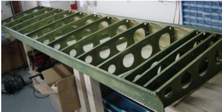
Basic or Primary Wing Structure; main and rear spars joined to middle/main ribs with zinc chromate primer.
