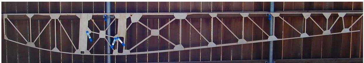
Fuselage side structure with truss cross bracing and gussets for strengthening
