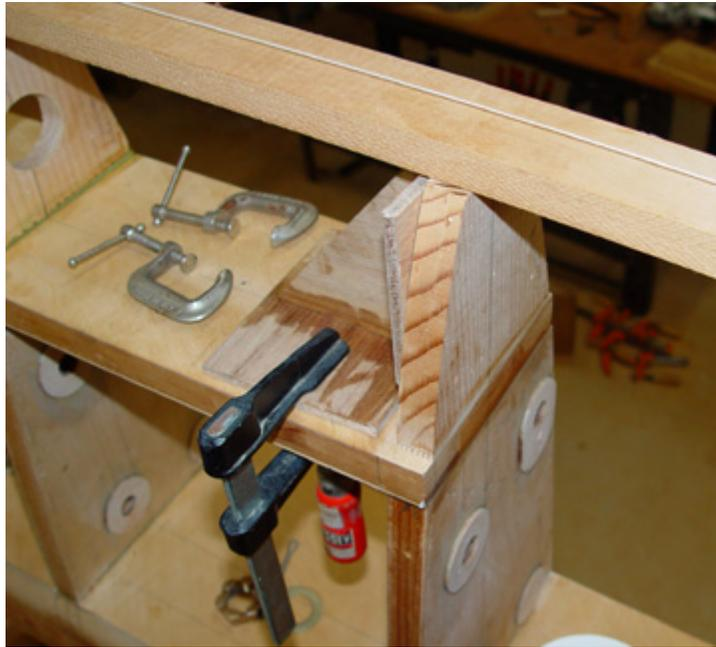
Spar and leading edge rib joining
