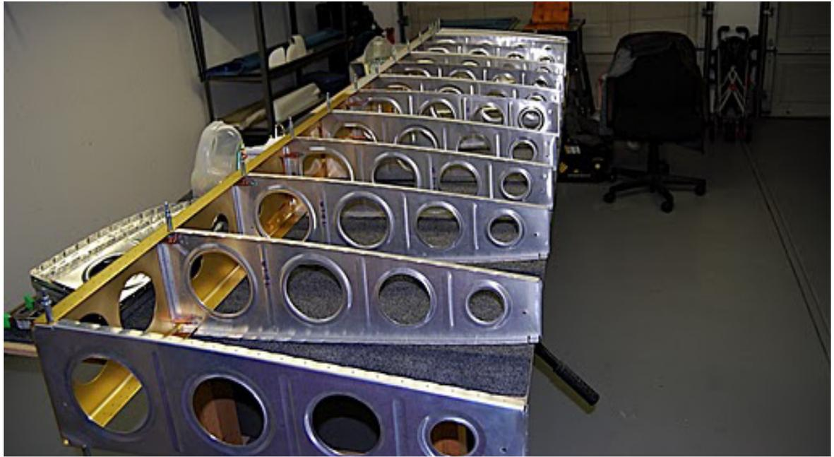
Main Spar with middle ribs attached.
