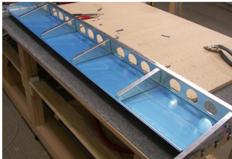
Conventional Spar and Rib Construction. Traditional spar at top, bottom skin is folded at rear to form a faux rear spar providing an attach point for ribs trailing edge .
