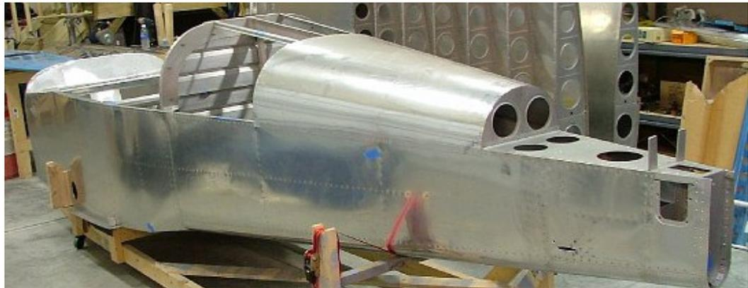
Quick build Fuselage out of the crate.
