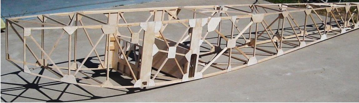
Basic wood fuselage internal structure
