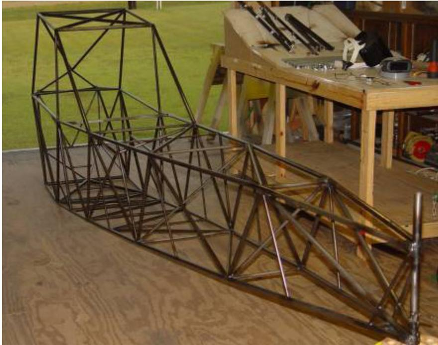
Steel Tube Fuselage prefabricated at the factory.
