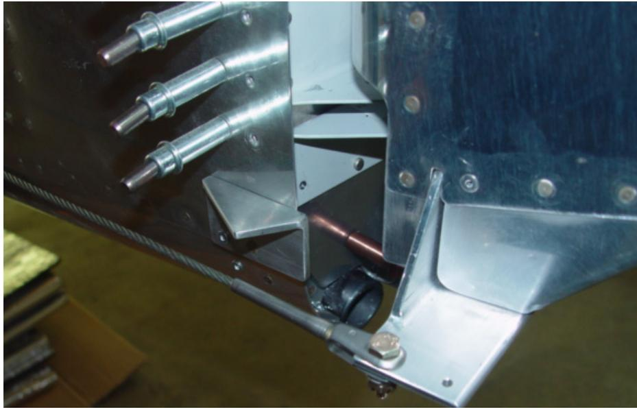
Rudder Cable attached to Rudder Horn
