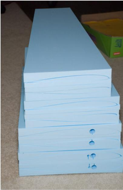
The foam material for the individual aircraft components may come out of the box like this photo to the left, in which case the builder would have to cut and shape the foam into the correct finished contour and form. Most composite kits provide the type of foam cores as shown below, with the foam cores properly shaped and sized, ready for application of fiberglass cloth and resin.
