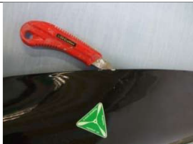
Delaminated composite shell on the trailing edge
