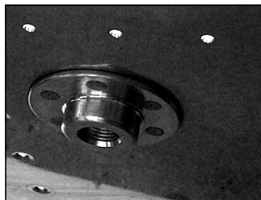
Fig.7-11. The VA-112 drain flange riveted to the outside of the tank skin.
