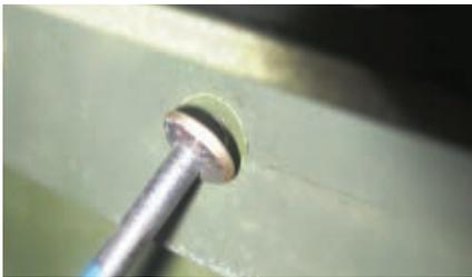
links to the original Navy method at [www.SportAviation.org](http://www.SportAviation.org).) Ken simplified the Navy method by eliminating the second step of drilling just through the head with a larger drill. He found that drilling down the center was sufficient to allow the head to be snapped off on the rivets he was working with. On some larger rivets you may need to perform the extra step of drilling through the head, using a drill the same size as the rivet diameter.
