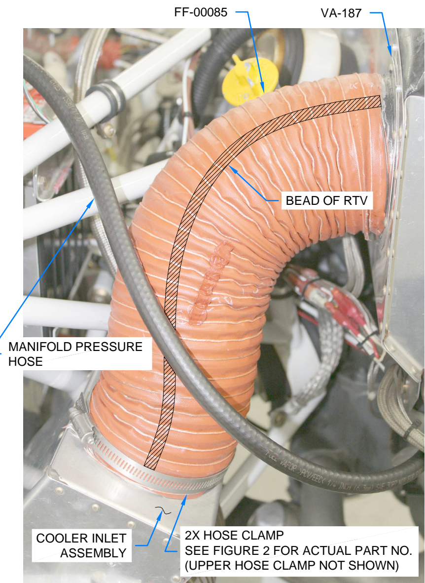
FIGURE 3: CONNECT SCAT DUCT (TRI-GEAR - RIGHT SIDE VIEW)
