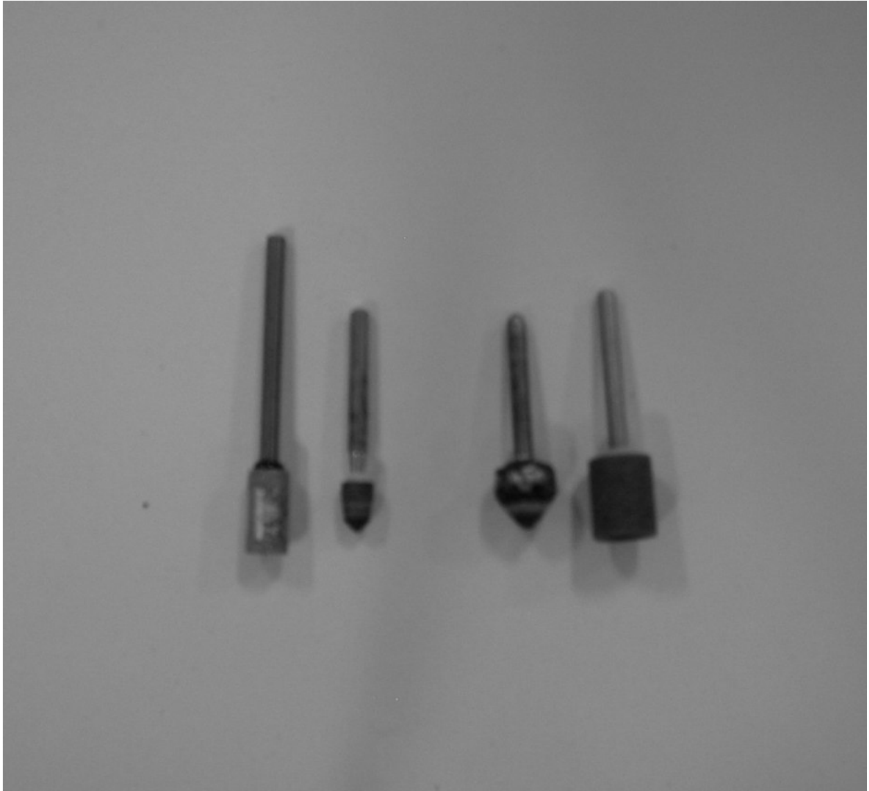
The tools are made from Dremel stone bits like these.
