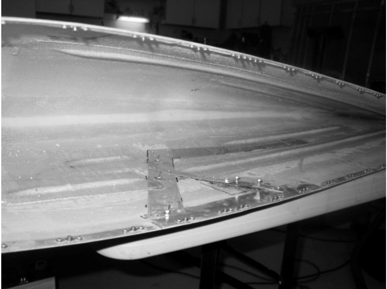
The Archer antenna is mounted and the dowels installed.
