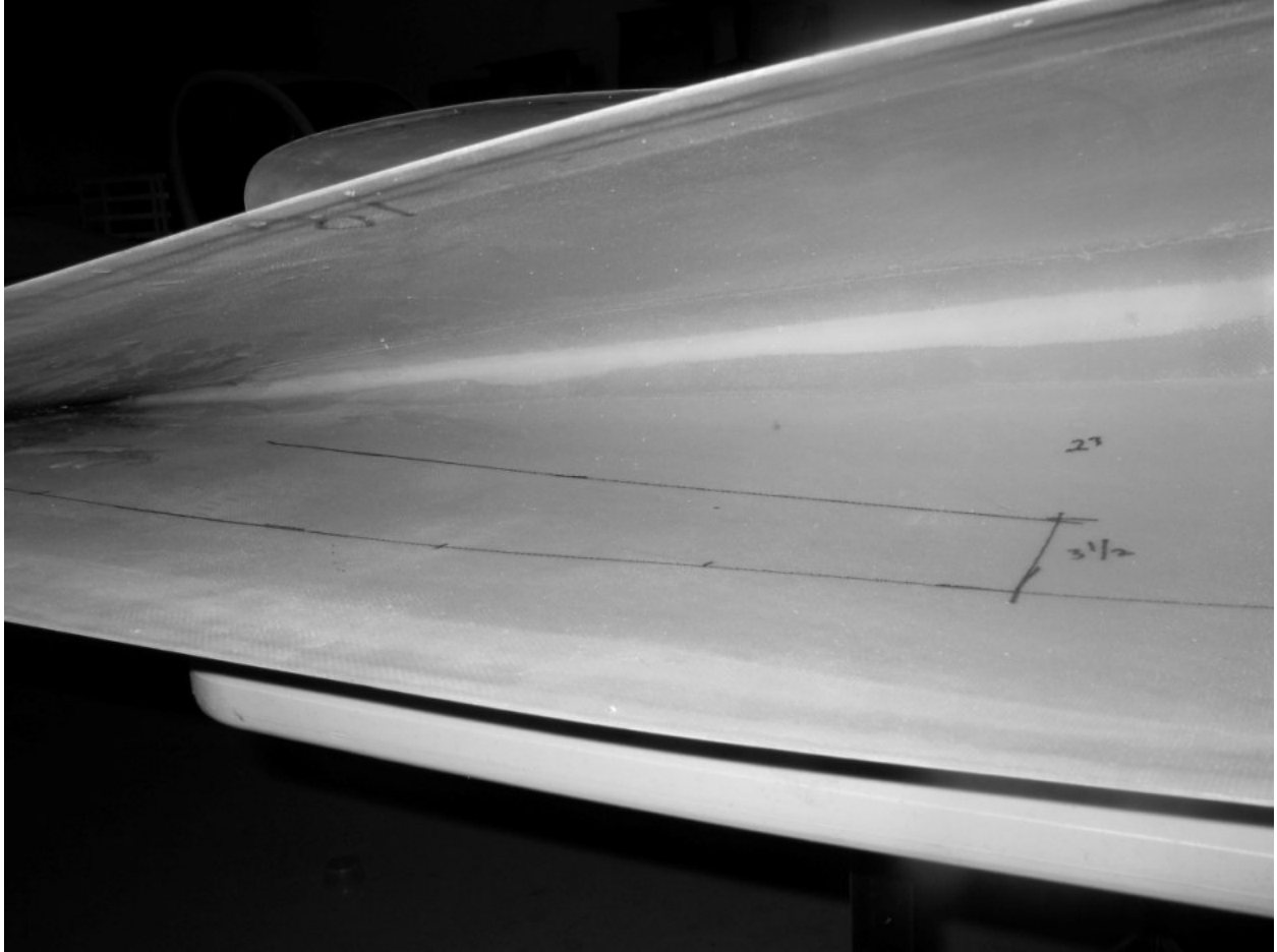
The location has been transferred to the inside of the tip, top and bottom.
